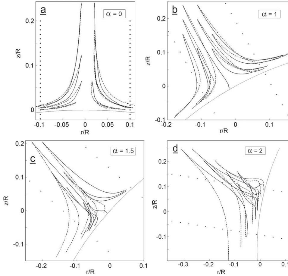
**Figure 10.** Particle trajectories for approach velocity  $V_a$  equal to  $3.5 \text{ mm s}^{-1}$  (dashed lines) and  $10 \text{ mm s}^{-1}$  (full lines). Frontal and oblique approach (particle diameter:  $280 \mu\text{m}$ ): (a)  $\alpha = 0$ , (b)  $\alpha = 1$ , (c)  $\alpha = 1.5$ , (d)  $\alpha = 2$ .
