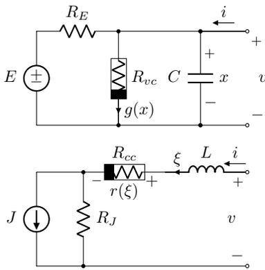
Fig. 2. Basic prototype circuits of a current-driven (above) and a voltage-driven (below) 1-passive circuit. The resistors  $R_{vc}$  and  $R_{cc}$  are voltage-controlled and current-controlled resistors respectively.
