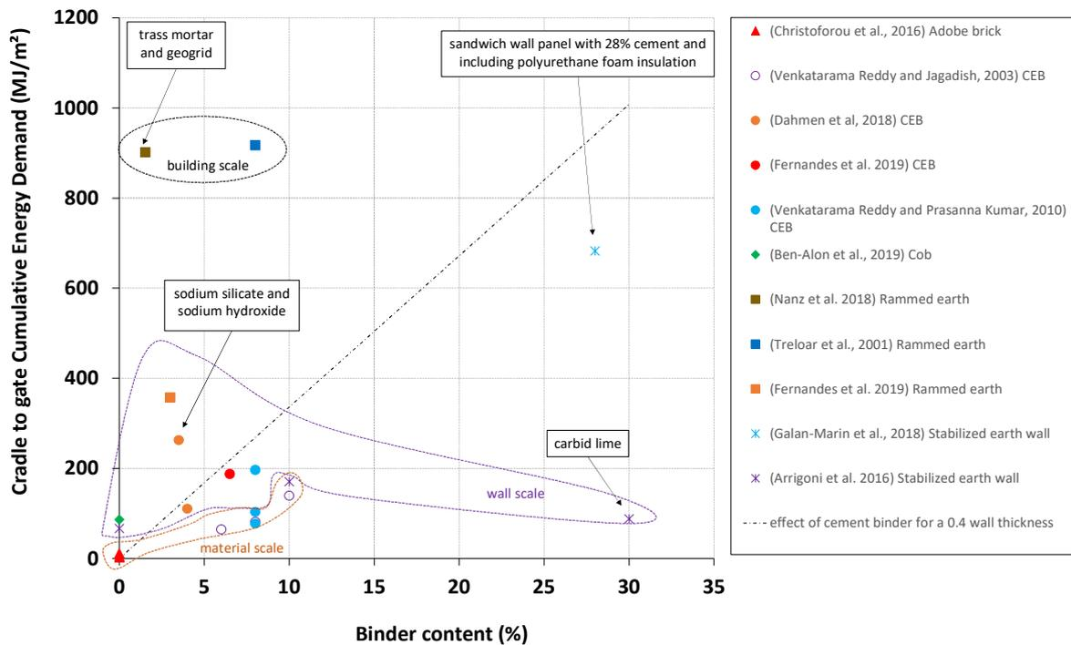
Figure 8-2. Influence of binder content on the cradle to gate Cumulative Energy Demand - shape is linked to construction technique: ○ CEB, □ Rammed earth, ◇ Cob, \* Stabilized earth wall, △ Adobe – unless indicated otherwise, binders are cement or lime.
