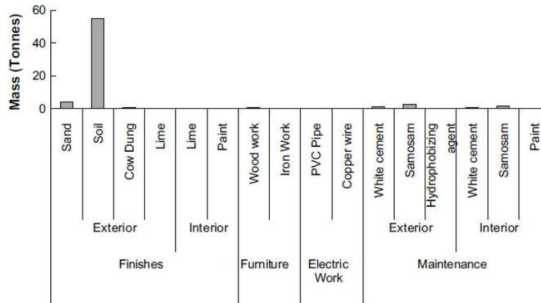
Figure A8- 4. Masses of materials for life phases of an adobe house in India (Shukla et al., 2009)
