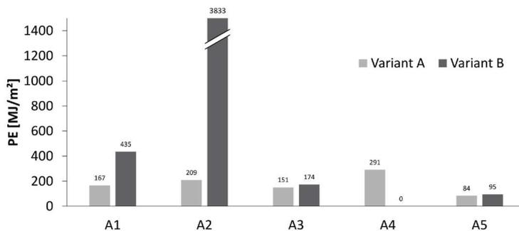
Figure A8- 3. Primary energy demand for the two variants studied - transports correspond to A2 and A4 stages (Nanz et al., 2018)
