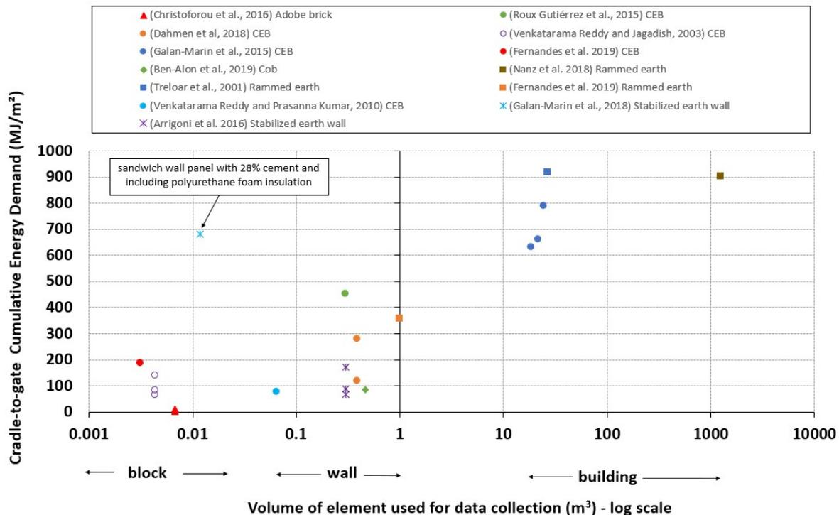
Figure 8- 3. Influence of scale used for data collection – shapes of plots are linked to the construction technique: ○ CEB, □ Rammed earth, ◇ Cob, \* Stabilized earth wall, △ Adobe
