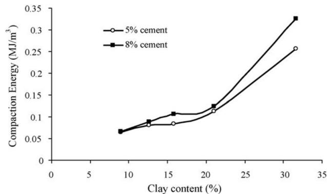
Figure A8- 2. Compaction energy for experimental wallettes according to clay and cement contents (Venkatarama Reddy and Prasanna Kumar, 2010).
