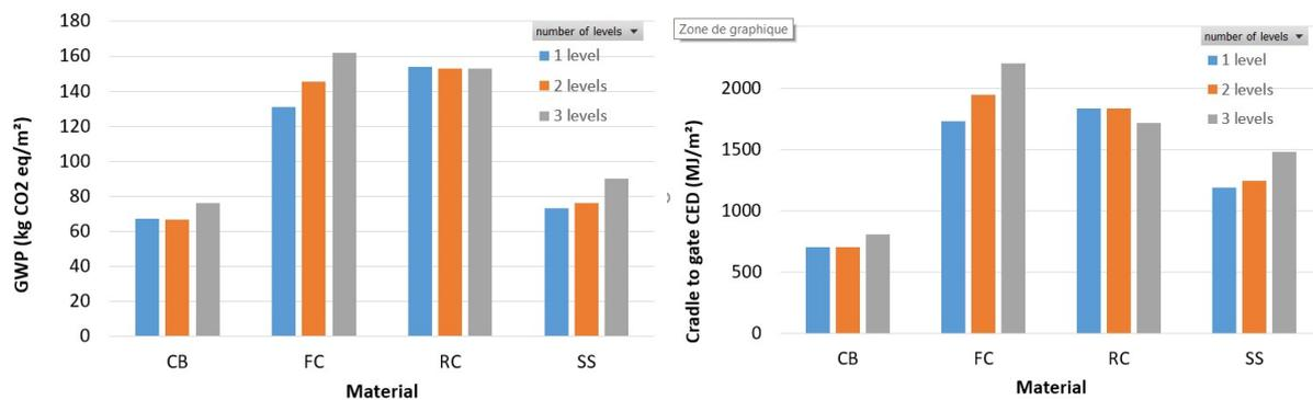
Figure 8- 4. Global Warming Potential (GWP100) and Cumulative Energy Demand (CED) for the same building, according to the number of levels, after (Galan-Marín et al., 2015b) – CB: concrete block masonry, FC: fire clay brick masonry, RC: reinforced concrete and SS: stabilized earth block masonry
