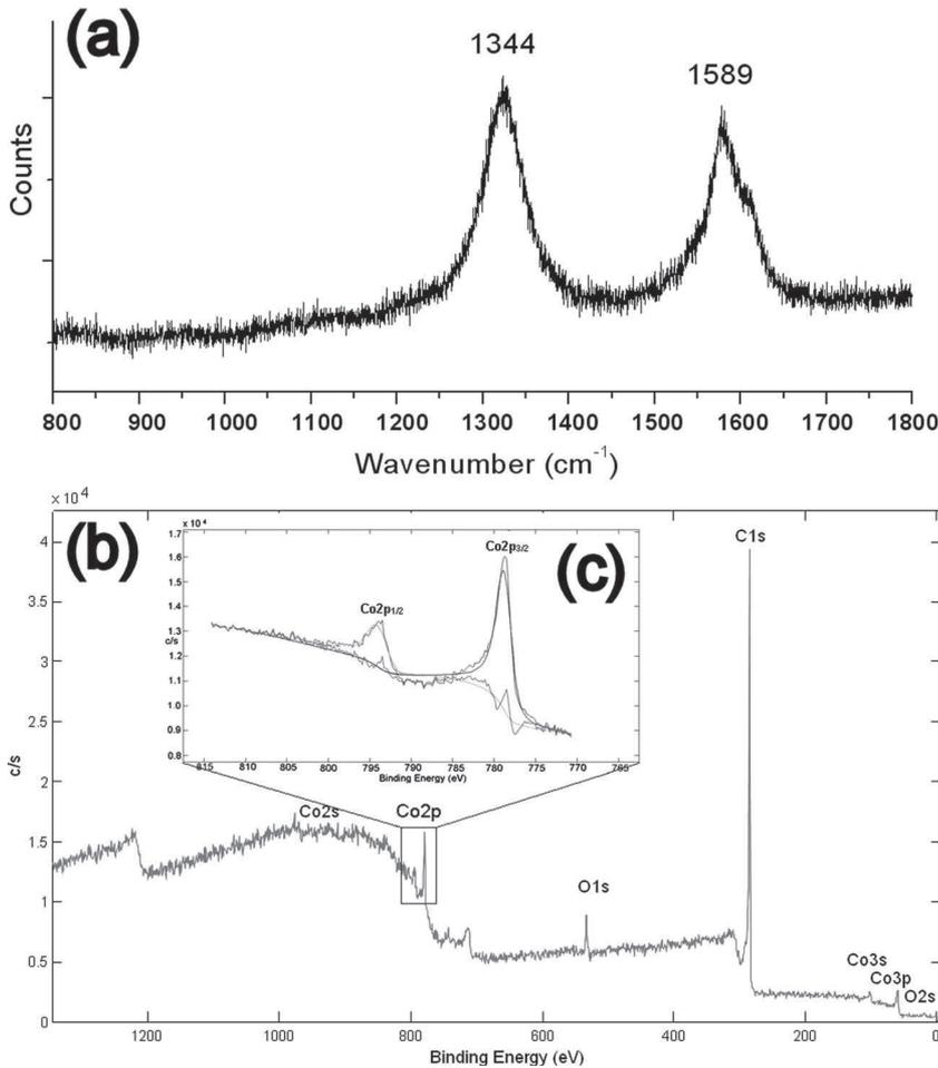
**Figure 2.** a) Raman spectra of Co@C nanoparticles exhibiting two bands (D at 1344 cm<sup>-1</sup> and G at 1589 cm<sup>-1</sup>); b) Normalized XPS survey spectrum; c) Co2p spectrum of Co@C nanoparticles after HCl treatment.
