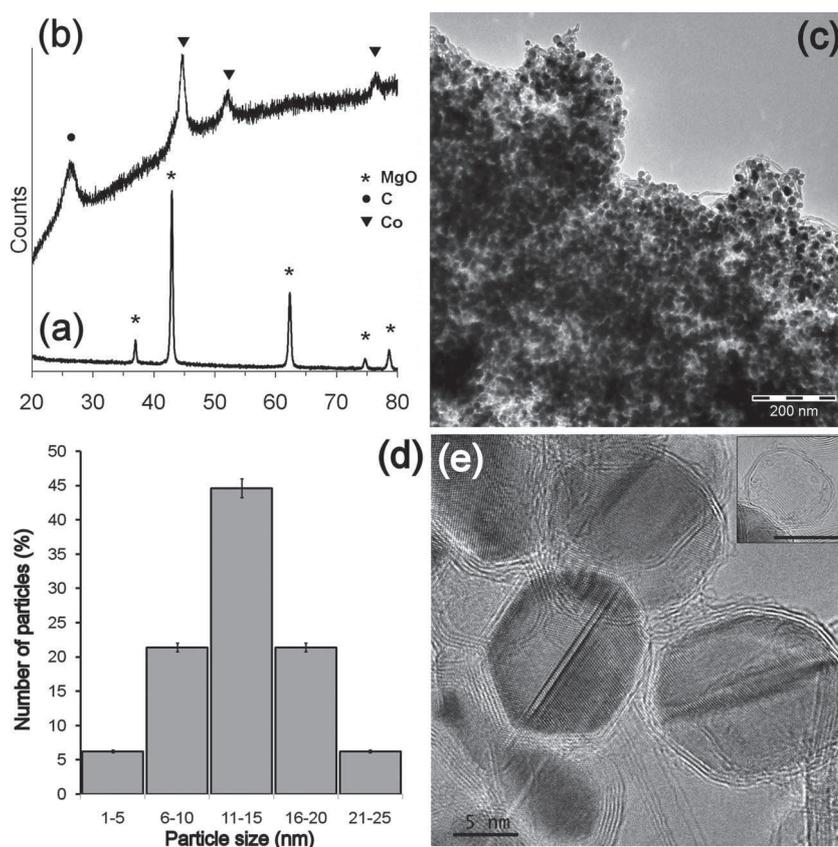
**Figure 1.** XRD patterns of a) C-Co-MgO nanocomposite powder and b) Co@C nanoparticles after HCl treatment; c) Low-magnification TEM image of Co@C nanoparticles after HCl treatment of the C-Co-MgO composite powder; d) particle size distribution of Co@C nanoparticles. e) HRTEM images of Co@C nanoparticles where the (fcc)-Co lattice is clearly visible, as well as the graphitic carbon shells. Inset (scale bar is 5 nm) shows empty carbon shells (metal removed);
