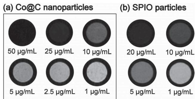
**Figure 4.**  $T_2$ -weighted MR contrast images: a) Co@C nanoparticles in solid phantoms, b) super-paramagnetic iron oxide (SPIO) particles in solid phantoms.  $T_2$ -weighted multi-slice multi echo (MSME) sequence is used with a pulse repetition time (TR) of  $2000 \text{ ms}$ , flip angle of  $180^\circ$ , echo time (TE) of  $30 \text{ ms}$  and slice thickness of  $2 \text{ mm}$ .
