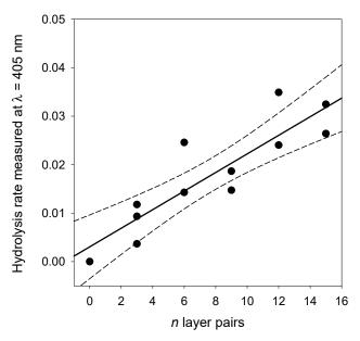
**Figure 11.** Evolution of the hydrolysis rate of  $(PAH-PDA@ALP)_n$  films as a function of the number of deposited layer pairs. The solid line corresponds to a linear regression of the data points, whereas the dashed lines correspond to the limit of the 95% confidence interval.
