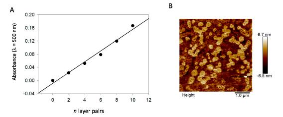
**Figure 9.** Incorporation of PDA@ALP nanoparticles in layer-by-layer films. (**A**) Evolution of the absorbance at  $\lambda = 500$  nm (where PAH does not absorb light) of (PAH-PDA@ALP)<sub>n</sub> films with the number of deposited layer pairs, *n*. (**B**) Film morphology of a (PAH-PDA@ALP)<sub>6</sub> film as investigated by means of contact mode AFM.
