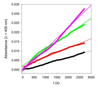
**Figure 10.** Enzymatic kinetics for (PAH-PDA@ALP)*n* films put in contact with a 20-fold diluted PNP solution as a function of the number of deposited layer pairs: n = 3 ( $-\bullet-$ ), n = 6 ( $-\bullet-$ ), n = 12 ( $-\bullet-$ ), and n = 15 ( $-\bullet-$ ). The data points correspond to the experimental data, whereas the solid lines correspond to linear regressions of the data.
