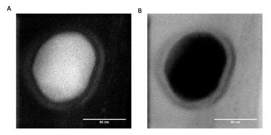
**Figure 3.** High-resolution STEM images acquired simultaneously in (**A**) high-angle annular dark field and (**B**) bright field modes of PDA@ALP nanoparticles obtained after 6 h of oxidation of a 10 mM dopamine solution + 1 mg·mL<sup>-1</sup> ALP in the presence of 20 mM NaIO<sub>4</sub>.
