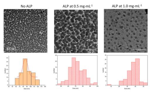
**Figure 2.** (**Top**) Representative TEM micrographs of polydopamine nanoparticles produced after 6 h of oxidation in the presence of 20 mM NaIO<sub>4</sub> from the dopamine solutions (10.6 mM) after the subsequent dialysis against Tris buffer, as a function of the added concentration in ALP. (**Bottom**) Size distribution of the particles obtained by analyzing 100 particles.
