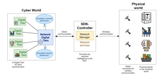
Figure 3. Digital Twin Networking based architecture for industry 4.0.
