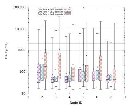
Figure 8. Packet Delay—Minimal TSCH.
