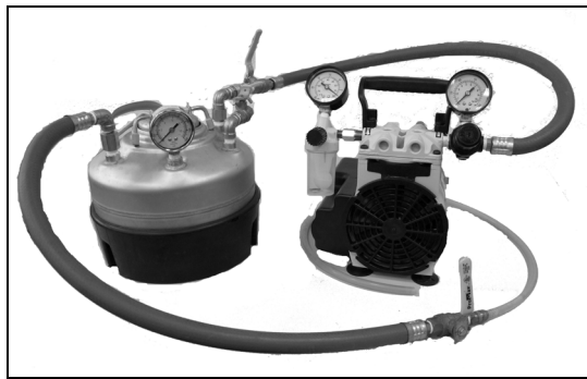
Fig. 1. Microbubble generation system based on aeroflotation
