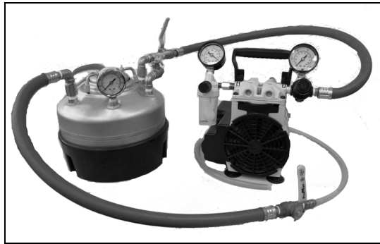
Fig. 1. Microbubble generation system based on aeroflotation
