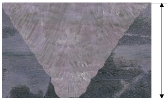
Figure 5: Macrograph of GTAW weld
