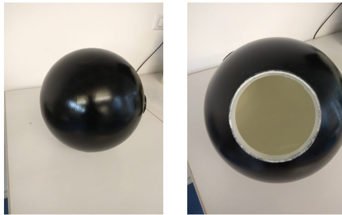
Figure 9. Painted integrating spheres: white inside and black outside
