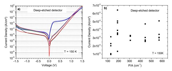
**Figure 11.** Deep-etched photodetectors: (**a**) dark current density voltage characteristics performed on different detector sizes at 150 K; (**b**) dark current density value as a function of the perimeter to area ratio, extracted at V = -400 mV.
