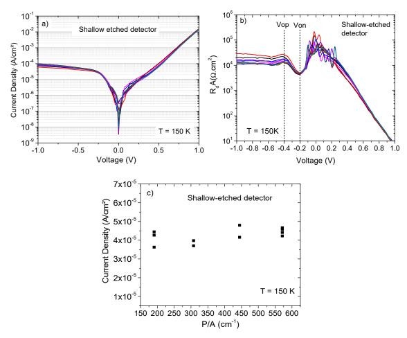
**Figure 5.** Shallow-etched photodetectors: (a) dark current density voltage characteristics performed on different detector sizes at 150 K; (b) differential Resistance Area product ( $R_dA$ ) product as a function of the voltage at 150 K; (c) dark current density value as a function of the perimeter to area ratio (P/A), extracted at  $V_{op} = -400$  mV.
