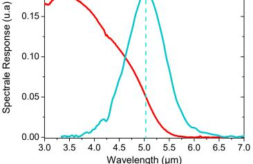
**Figure 4.** InAsSb/InAs T2SL structure: photo-response (PR) spectrum at -400 mV and photoluminescence (PL) measurement performed at 150 K.
