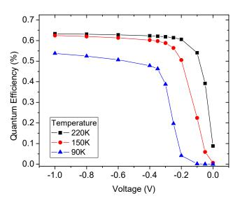
**Figure 9.** Quantum efficiency (QE) at  $\lambda = 3.4 \mu m$  of the deep-etched photodetector for T = 90, 150 and 220 K versus applied bias. At T = 150 K, the QE is equal to 60 % at the operating bias (V = -0.4 V).
