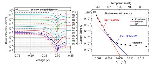
**Figure 8.** (a) Dark current density measured for a shallow-etched device with a 210  $\mu$ m diameter at different temperatures; (b) temperature dependence of dark current density at -0.4 V.
