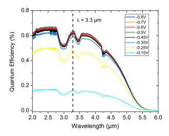
**Figure 7.** Front-side illuminated spectral quantum efficiency taken at T = 150 K and under different biases of the shallow-etched circular mesa photodetectors with diameter size including the additional lateral diffusion length.
