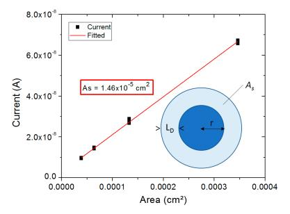
additional surface area created by the important lateral diffusion length, a correction in the photodetector area is necessary to obtain the real electric performance.
