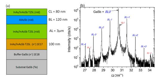
**Figure 1.** (a) Stacking of the XBn InAs/InAsSb T2SL structure grown by MBE on GaSb substrate. (b) HR-XRD pattern of the T2SL detector structure. The lattice mismatch with the GaSb substrate is -354 ppm.
