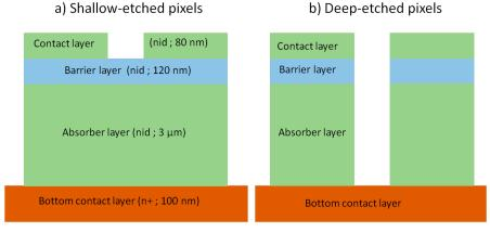
Figure 3. Schematic view of shallow-etched (a) and deep-etched (b) pixels.
