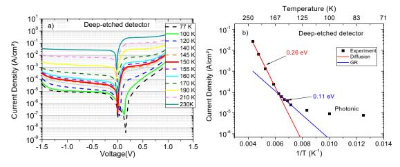
**Figure 10.** (a) Dark current density characteristics measured for a deep-etched device (mesa size 210  $\mu$ m) at different temperatures from 77 to 230 K; (b) temperature dependence of dark current density at -0.4 V.
