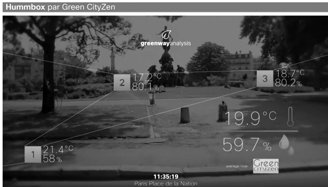
Figure 7. The Green CityZEN enterprise has recently experimented with digital sensors to monitor soil moisture, soil temperature, rainfall and wind speed of public green spaces, in order to adjust watering routines at Place de la Nation in Paris. (Source: © Green CityZen, 2017. https://www.youtube.com/watch?v=rIXsY9h7eyw )
