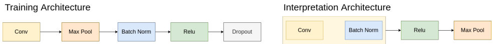
Figure 1: Modification of the ordering of the network inner layers. Left: Order for training and test. Right: Order for interpretation. Weights of each layer remain unchanged. For interpretation, Convolution and Batch Norm layers are merged into a functionally equivalent convolutional layer. A mathematical justification is given in the supplementary material.
