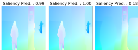
Figure 2: Starting from the optical flow (left), we replace the flow in the selected regions by inpainting. When the tree-trunk region in the foreground is ablated, the frame is still classified as dynamically salient (middle). In contrast, ablating regions of the two moving people switches the frame as non salient (right). See the prediction score above each frame.
