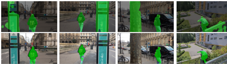
Figure 3: Extracted salient masks, superimposed on original images, on three examples from our dataset and one from DAVIS2016 (Parkour). Top row : results from [26] using the available code and model (without the postprocessing step). Bottom row : corresponding results using our method (NIMS). CIS [26] detects the foreground static object due to parallax motion, while our method successfully discards it. The sequence of the third example is available in the Supplementary Material.
