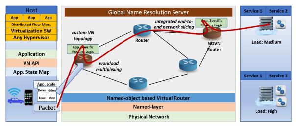
Fig. 5. Overview of an application-aware Full Stack Virtualization architecture
