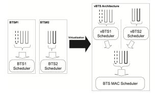
Fig. 2. Service flow abstractions on a virtualized base station
