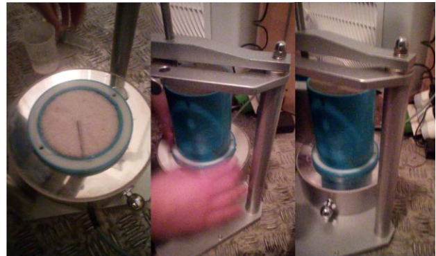
Figure 1. Illustrations of the experimental setup: a) Container fixed in a frame (left); Placing soil sample in the lower area (centre). Soil sample in cylinder (right)
