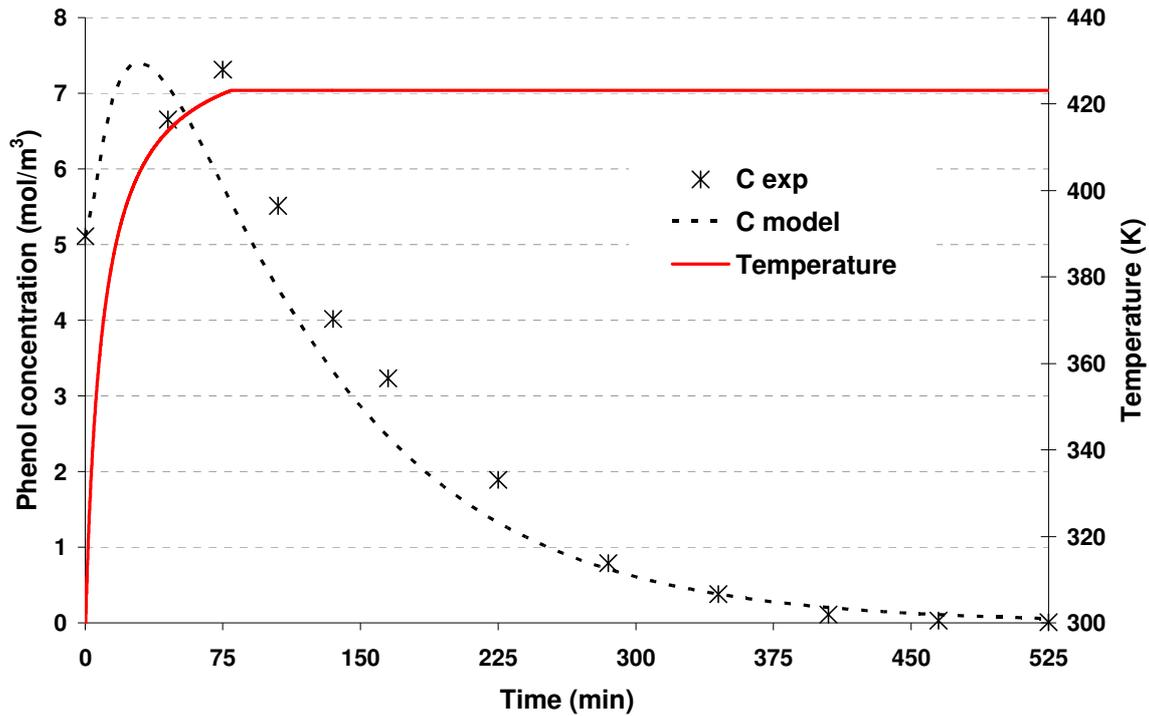
Figure 6. Evolution of temperature and phenol concentration in the mixed tank during last oxidation step –  $w_{AC} = 7.23 \text{ g}$  -  $Q_L = 2.44 \text{ L.h}^{-1}$  -  $Q_{air} = 30 \text{ NL.h}^{-1}$  -  $C_0 = 5.3 \text{ mol.m}^{-3}$  -  $P = 50 \text{ bar}$  -  $T = 423.15 \text{ K}$ : experimental and simulated profiles.
