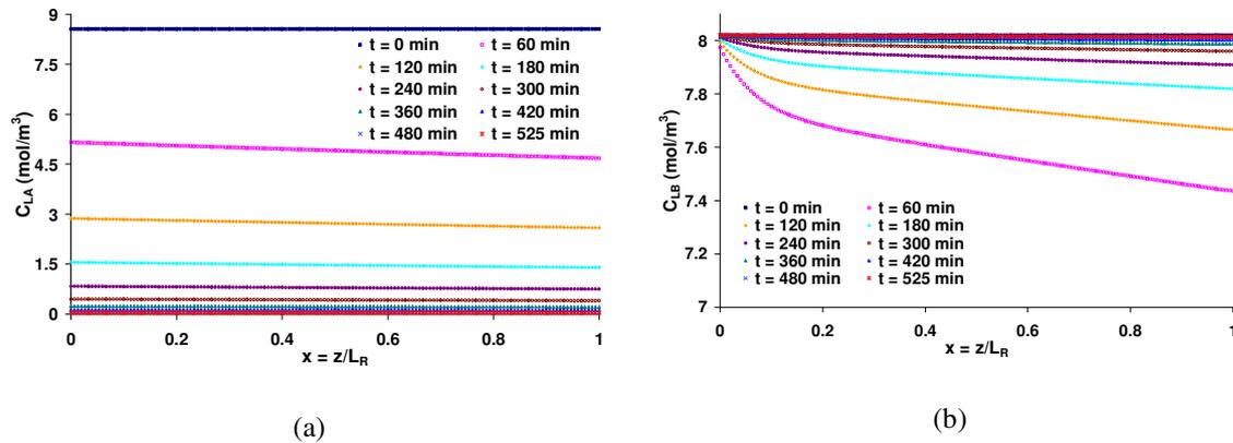
Figure 5: Axial concentration profiles of phenol (a) and oxygen (b) in the FBR (assuming constant temperature) –
