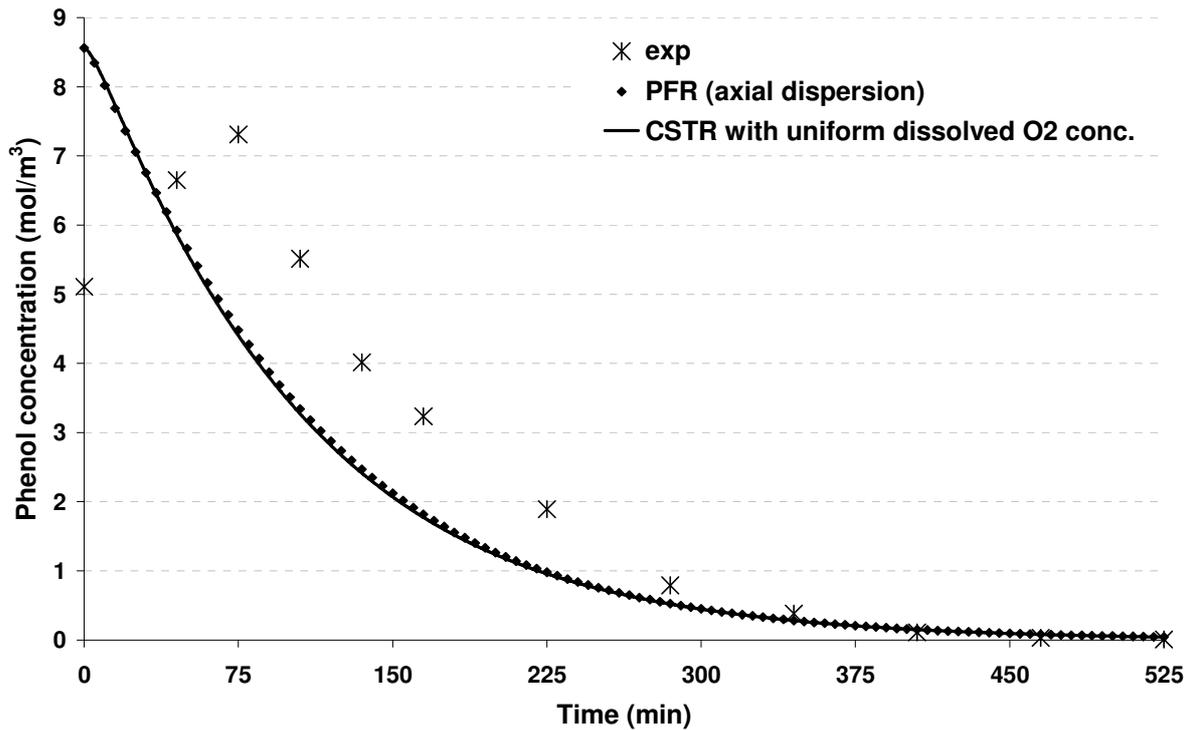
Figure 4. Evolution of phenol concentration in the mixed tank during last oxidation step –
