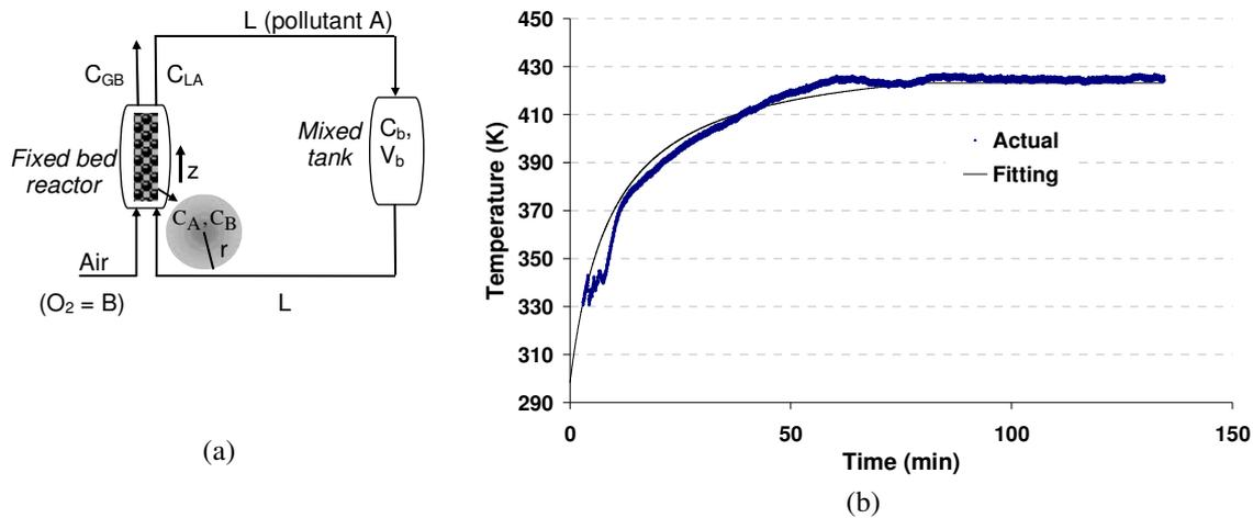
Figure 3. (a) Simplified scheme of AD-OX set-up, (b) fitting of experimental outlet temperature during heating period.
