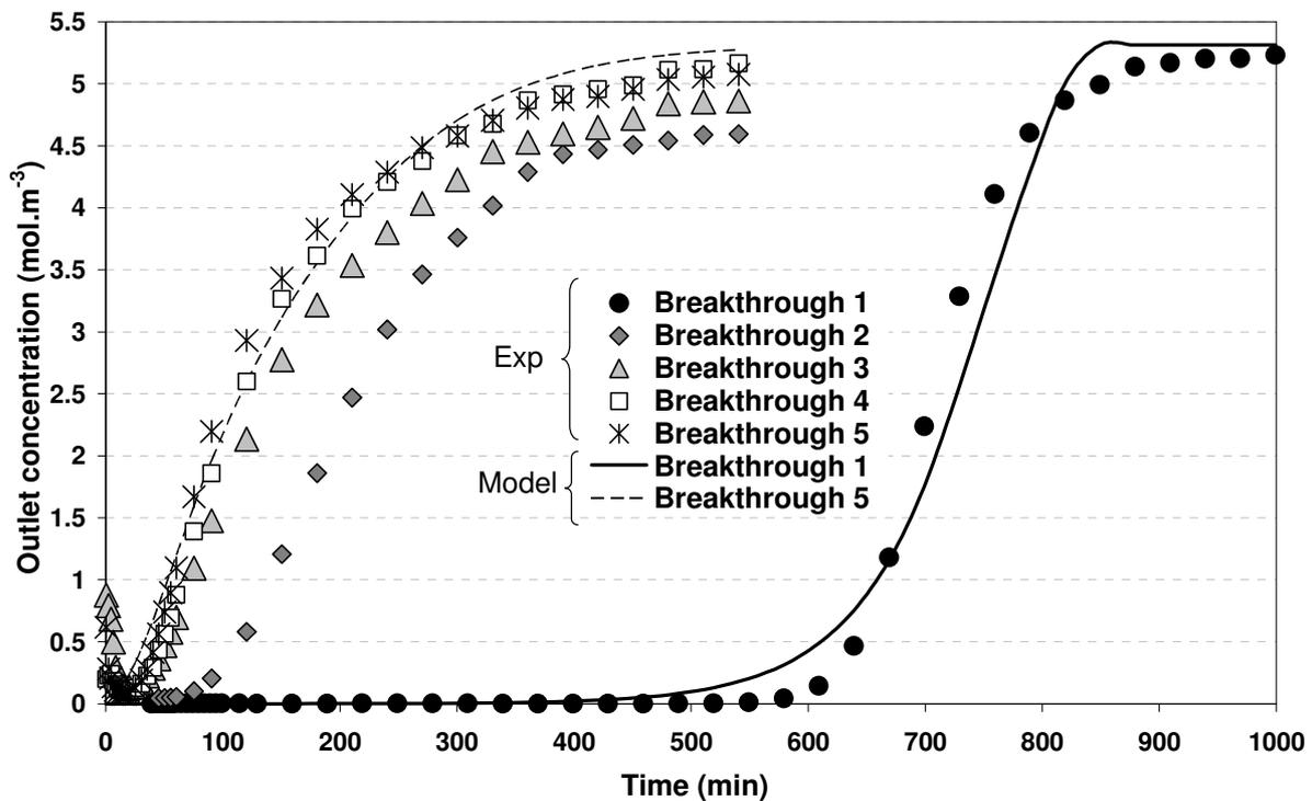
Figure 2. Successive breakthrough curves on PICA F22 (phenol adsorption) -  $Q_L = 0.23 \text{ L.h}^{-1}$  -  $C_{\text{feed}} = 5.3 \text{ mol.m}^{-3}$  -  $m_{\text{AC}} = 7.23 \text{ g}$  -  $T = 298.15 \text{ K}$ : experimental and simulated profiles.
