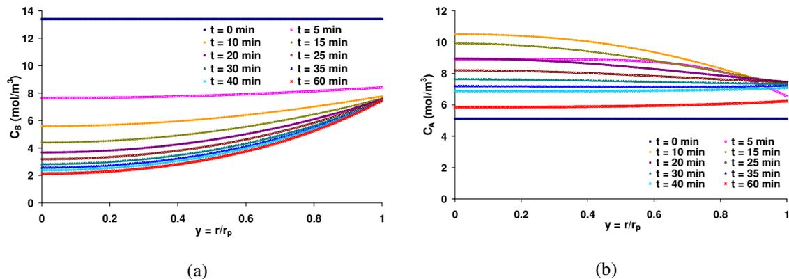
Figure 7. Radial concentration profiles of oxygen (a) and phenol (b) in the AC pellet –  $w_{AC} = 7.23 \text{ g}$  -  $Q_L = 2.44 \text{ L.h}^{-1}$  -  $Q_{air} = 30 \text{ NL.h}^{-1}$  -  $C_0 = 5.3 \text{ mol.m}^{-3}$  -  $P = 50 \text{ bar}$  -  $T = 423.15 \text{ K}$ .
