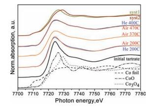
**Figure 3.** Co K-edge XANES of Co-doped calcium tartrate, heated in air at 200 °C, 370 °C, and 470 °C or in He at 200 °C and 400 °C and products of final decomposition of the tartrate in inert atmosphere (syst1) or in air (syst2) in comparison with the spectra of reference samples Co foil, CoO, and Co<sub>3</sub>O<sub>4</sub>.
