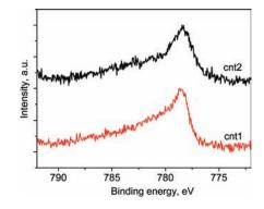
Figure 7. XPS spectra of Co  $2p_{3/2}$  level for CNT samples synthesized by  $C_2H_5OH$  decomposition over syst1 (cnt1) and CH<sub>4</sub> decomposition over syst2 (cnt2).
