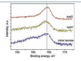
**Figure 4.** XPS spectra of the Co  $2p_{3/2}$  level for Co-doped calcium tartrate and products of its decomposition in Ar atmosphere (syst1) or in air (syst2).
