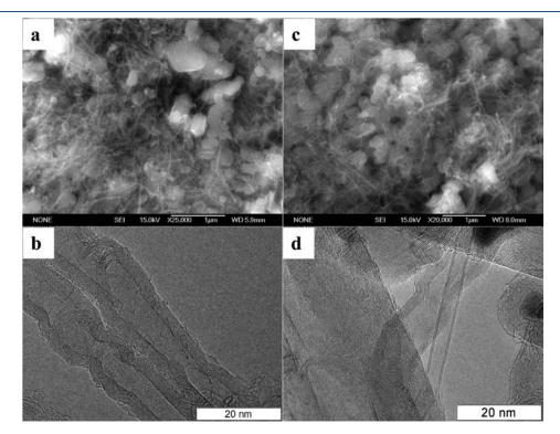
Figure 5. SEM (a) and HRTEM (b) image of sample produced by  $C_2H_5OH$  decomposition over syst1 at 800 °C. SEM (c) and HRTEM (d) image of sample produced by CH<sub>4</sub> decomposition over syst2 at 1000 °C.
