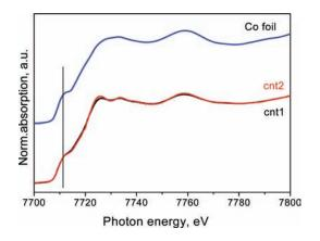
Figure 6. Co K-edge XANES of CCVD products of  $C_2H_5OH$  decomposition over syst1 (cnt1) and CH<sub>4</sub> decomposition over syst2 (cnt2) in comparison with the spectrum of Co foil.
