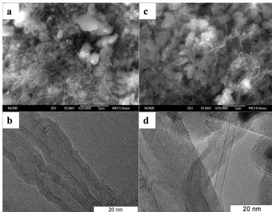
**Figure 5.** SEM (a) and HRTEM (b) image of sample produced by  $C_2H_5OH$  decomposition over syst1 at 800 °C. SEM (c) and HRTEM (d) image of sample produced by  $CH_4$  decomposition over syst2 at 1000 °C.
