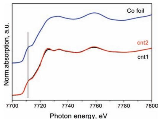
**Figure 6.** Co K-edge XANES of CCVD products of  $C_2H_5OH$  decomposition over syst1 (cnt1) and  $CH_4$  decomposition over syst2 (cnt2) in comparison with the spectrum of Co foil.
