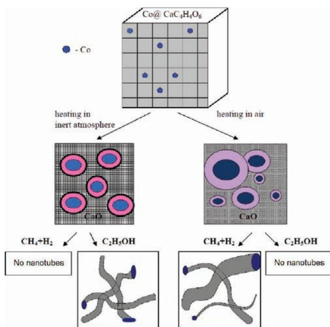
**Figure 8.** Scheme of transformation of Co-doped calcium tartrate under heating in inert atmosphere or in air and of the CaO-supported metallic nanoparticles in the CCVD process utilizing specific feedstock (ethanol or CH<sub>4</sub> + H<sub>2</sub>).
