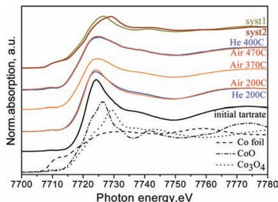
**Figure 3.** Co K-edge XANES of Co-doped calcium tartrate, heated in air at 200 °C, 370 °C, and 470 °C or in He at 200 °C and 400 °C and products of final decomposition of the tartrate in inert atmosphere (syst1) or in air (syst2) in comparison with the spectra of reference samples Co foil, CoO, and  $\text{Co}_3\text{O}_4$ .
