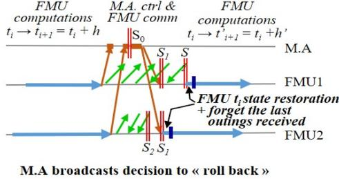
Figure 5: Overlapped orchestration mode with Rollback.
