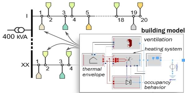
Figure 8: Ideas use-case, to model the thermal behavior and electricity consumption of 1000 buildings with 1042 FMUs.
