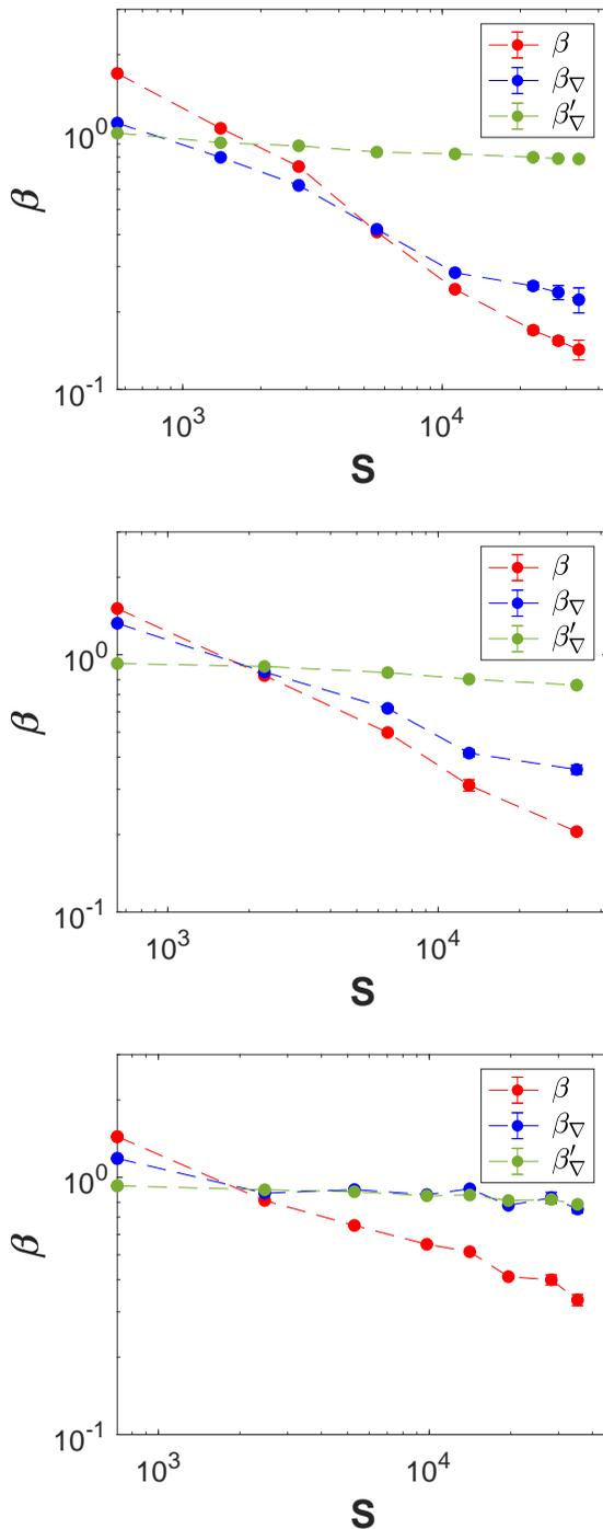
FIGURE 4. Lundquist-number dependence of three alternative definitions of  $\beta$  in cylinders with ellipticity (a)  $a = 1$ , (b)  $a = 1.2$ , (c)  $a = 1.4$ . Whereas the pressure based  $\beta$  is strongly decreasing with  $S$ , the gradient based value  $\beta'_{\nabla}$  is roughly constant.
