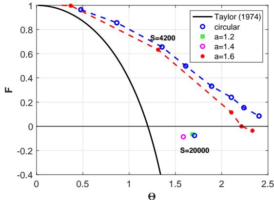
FIGURE 2. Field reversal parameter  $F$  as a function of the pinch parameter  $\Theta$  for cylinders with circular and elliptic cross-section. Also shown is Taylor's prediction (Taylor 1974) for reference.
