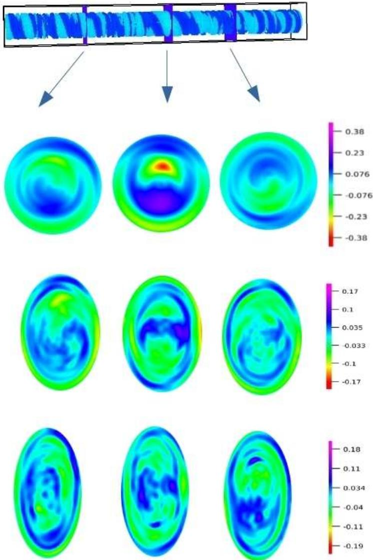
FIGURE 6. Poloidal cross-sections of the cylinder, illustrating the axial magnetic fluctuations at  $t = 9.8 \cdot 10^3 \tau_A$  for  $S \approx 2 \cdot 10^4$ . The geometries are a circle with radius  $a = 1$ , an ellipse with major semi-axis  $a = 1.2$  and one with  $a = 1.4$ .
