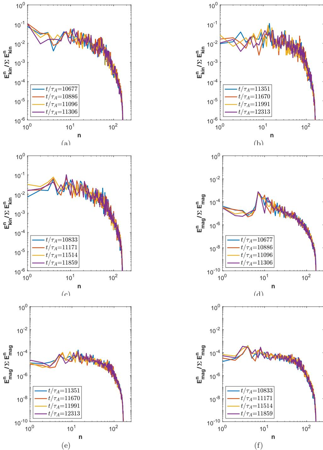
FIGURE 9. Axial mode spectra of kinetic energy fluctuations (top row) and magnetic fluctuations (bottom row) in cylinders with ellipticity (a,d)  $a = 1$ , (b,e)  $a = 1.2$ , (c,f)  $a = 1.4$ . Spectra are shown at four different time-instants during the statistically steady state. The Lundquist number is  $S \approx 2 \cdot 10^4$ .
