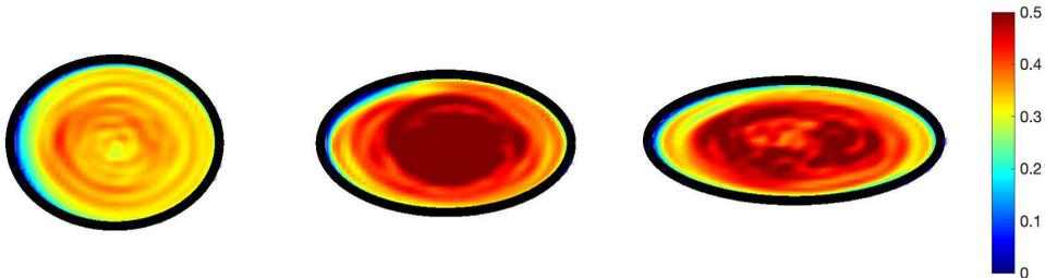
FIGURE 3. Instantaneous visualizations of the pressure field for  $S \approx 2 \cdot 10^4$  in cross-sections through the cylinders for the three different ellipticities. From left to right,  $a = 1$ ,  $a = 1.2$ ,  $a = 1.4$ .
