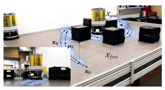
Fig. 1: Using a chance-constrained problem formulation, the proposed sequential convex programming algorithm efficiently plans safe trajectories despite nonlinear dynamics, nonconvex constraints, model uncertainty, and external disturbances.
