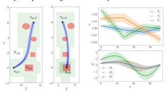
Fig. 3: Left: projections of the trajectory computed by (CC-SCP), avoiding all spherical and polygonal obstacles on-board the ISS. Right: 90% confidence intervals of the control input trajectory.
