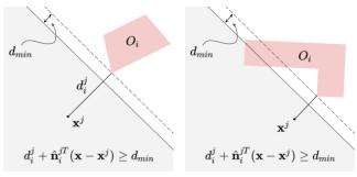
Fig. 5: Obstacle constraints convex reformulation using the signed distance function (21). On the left, this is conservative since the obstacle is convex. On the right, it is not.
