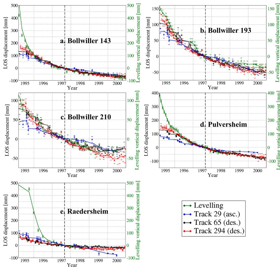
**Fig. 5.** Levelling and InSAR time series at the location of the five instrumented points by levelling from 1995 to 2000 (a-c. Bollwiler, d. Raedersheim., e. Pulversheim). The continuous lines show the displacements using a 2 month-long sliding window. The dotted line indicates the reference date 1997/09/03. Time series are shifted to a common zero based on the displacement difference linearly interpolated between the closest dates before and after the reference date.
