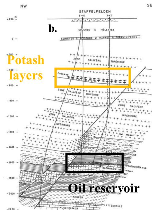
**Fig. 7.** Potential sources of surface displacements. a: Mean LOS velocity during ENVISAT period with the pumping sites (blue circles) and faults (black lines); b: Geological section across Staffelfelden (adapted from Sittler, 1972). The location of faults at depth has been projected at the surface. (For interpretation of the references to color in this figure legend, the reader is referred to the web version of this article.)
