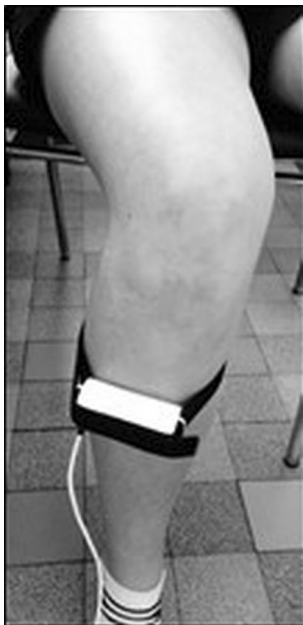
Fig. 2 Illustration of the vibratory device strapped on the tibialis anterior muscle belly
