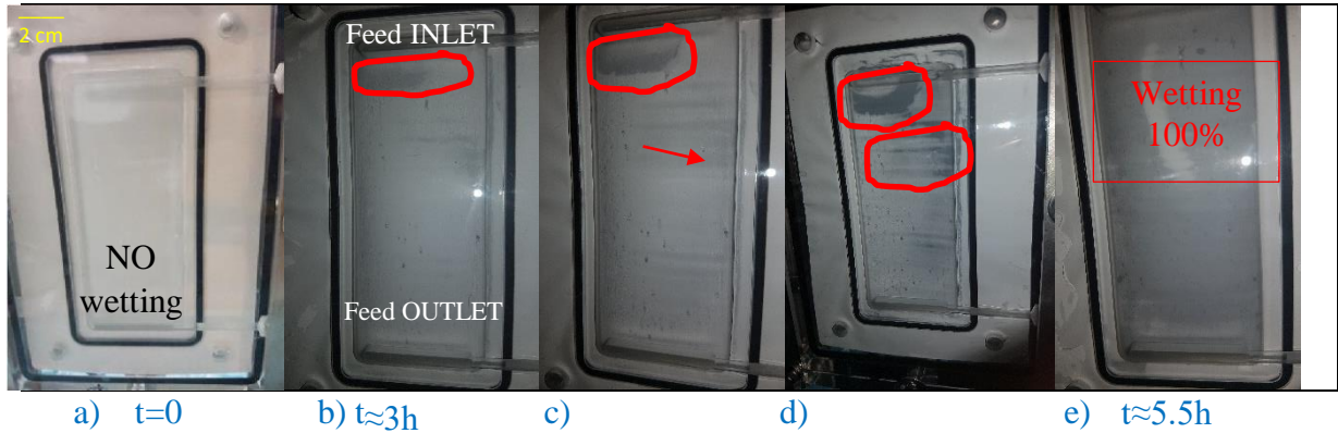
Figure 7: Visualization of the wetting phenomena with a porous PVDF membrane, from the feed inlet to the feed outlet. Feed: NaCl 10g/L + 1g/L SDS à 50°C. On the Fig. 7_b) and Fig. 7_c) the dark strips indicate some partial wetting.
