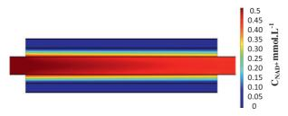
**Fig. 11.** Simulated concentration profile of NAD<sup>+</sup> in the reactor.  $[NAD^+]^\circ = 0.5 \text{ mmol L}^{-1}, \ [HCO_2^-]^\circ = 0.1 \text{ mol L}^{-1}, \ T = 38 \,^\circ\text{C}.$  Flow rate 63  $\mu\text{l min}^{-1}$ . Apparent diffusion coefficient  $D_a = 2.1 \times 10^{-11} \, \text{m}^2 \, \text{s}^{-1}$ .
