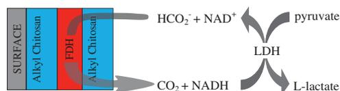
**Fig. 3.** Schematic representation of the enzymatic regeneration of NADH using formate dehydrogenase (FDH) coupled to a model enzymatic reaction, namely L-lactate synthesis from pyruvate catalyzed by L-lactate dehydrogenase. The enzyme was immobilized in an alkyl modified chitosan matrix according to a 'layer by layer' structure.
