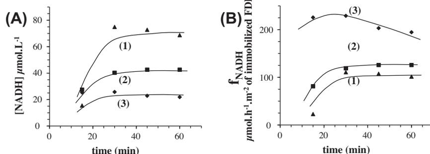
**Fig. 8.** Time dependence of the NADH produced for various volumetric flows. Inlet solution:  $\text{NAD}^+ 500 \mu\text{mol L}^{-1}$ ;  $\text{HCOO}^- 0.1 \text{ mol L}^{-1}$ ; phosphate buffer pH = 7.0;  $38 \text{ }^\circ\text{C}$ . (1) to (3) respectively 63, 127 and  $380 \mu\text{L min}^{-1}$ . Analyses were performed on the solution collected at the outlet of the reactor and cumulated for 15 min. (A): Outlet concentration of NADH; (B): production of NADH.
