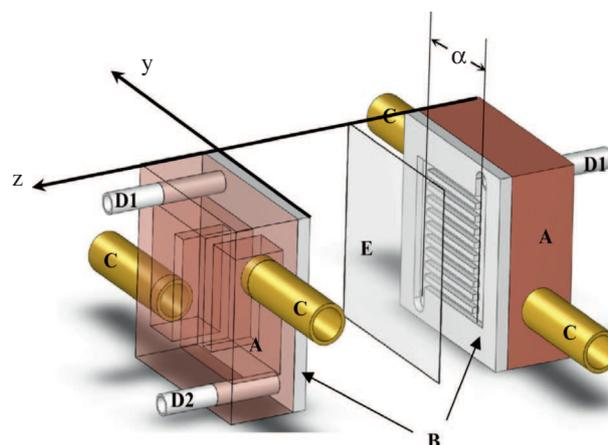
**Fig. 6.** Microstructured filter-press reactor. (A) Thermal exchanger; (B) Microstructured plate (containing 130 semi-cylindrical micro-channels of  $160 \mu\text{m}$  diameter) coated with immobilized FDH; (C) Inlet and outlet of heating fluid; (D1, D2) Reaction mixture outlet and inlet; (E) Ion exchange membrane (optional).
