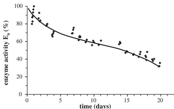
**Fig. 7.** Percentage of initial enzymatic activity ( $E_a$ ) as a function of the duration of the continuous operation. Inlet solution:  $[\text{NAD}^+]^0 = 0.5 \text{ mmol L}^{-1}$ ,  $[\text{HCOO}^-]^0 = 0.1 \text{ mol L}^{-1}$  in phosphate buffer pH = 7,  $Q = 63 \mu\text{L min}^{-1}$ ,  $T = 38 \text{ }^\circ\text{C}$ .
