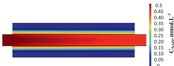
**Fig. 11.** Simulated concentration profile of  $\text{NAD}^+$  in the reactor.  $[\text{NAD}^+]^\circ = 0.5 \text{ mmol L}^{-1}$ ,  $[\text{HCO}_2^-]^\circ = 0.1 \text{ mol L}^{-1}$ ,  $T = 38^\circ \text{C}$ . Flow rate  $63 \mu\text{L min}^{-1}$ . Apparent diffusion coefficient  $D_a = 2.1 \times 10^{-11} \text{ m}^2 \text{ s}^{-1}$ .
