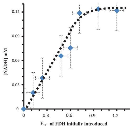
**Fig. 5.** Concentration of NADH produced at 38 °C by reaction (1) as a function of the quantity of initially introduced FDH ( $E_U$ ). Reaction duration 1 h; FDH immobilized in a 'butylchitosan macroporous polymer' coated at a microstructured plate, submitted to 5 washing process;  $[\text{NAD}^+]^0 = 0.5 \text{ mmol L}^{-1}$ ;  $[\text{HCOO}^-]^0 = 0.1 \text{ mol L}^{-1}$ .
