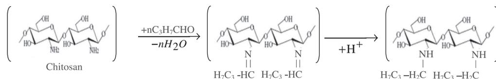
**Fig. 2.** Structure of chitosan and reaction scheme of its functionalization.
