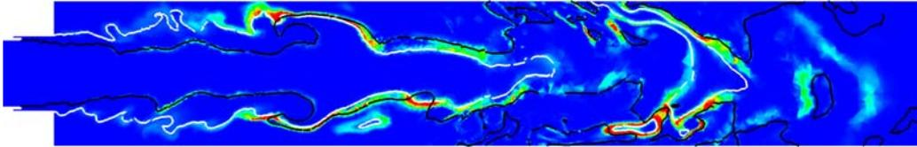
**Fig. 14** Longitudinal cut of heat-release rate field with stoichiometric (black) and  $T = 2000$  K (white) iso-contours.
