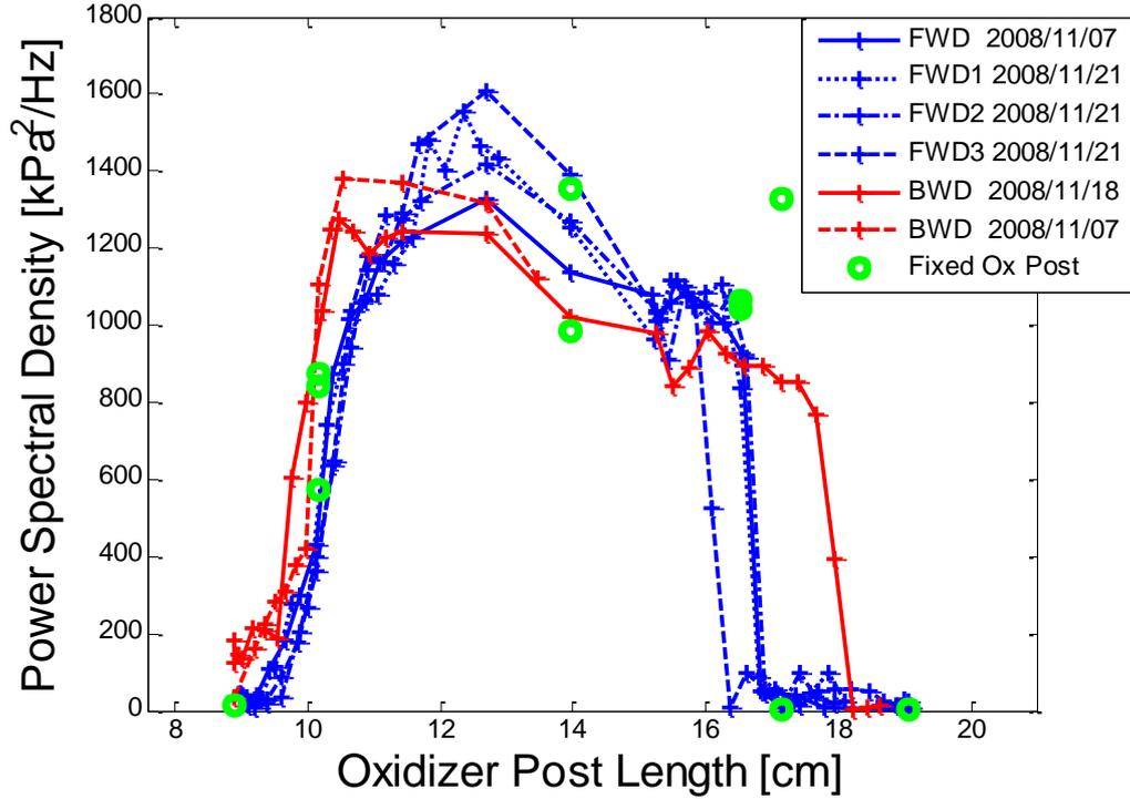
Fig. 4 Stability map of the CVRC experiment: power spectral density of the first mode versus  $L_{op}$ . The oxidizer translating shaft is either pushed forward, pulled backward or kept at a fixed position during the test.
