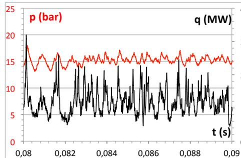
**Fig. 9 Pressure and heat release - Stable regime**
