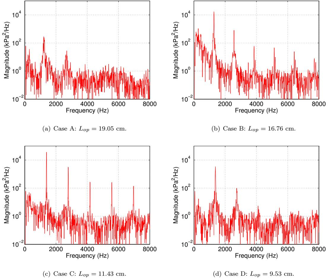
**Fig. 5 Power spectral density of the pressure signal at point P<sub>2</sub> in the experiment.**
