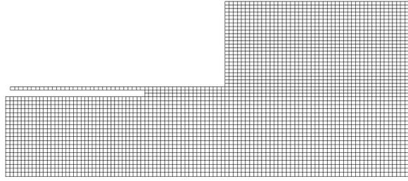
Fig. 6 Mesh - zoom on the combustion chamber entrance
