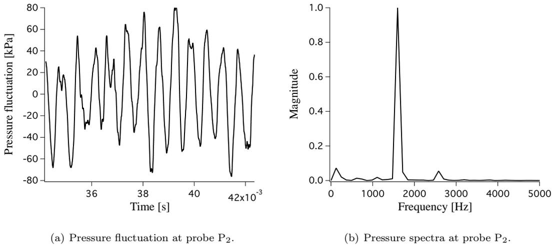
**Fig. 15** Pressure signal and spectra recorded at probe P<sub>2</sub>.
