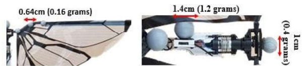
Figure 3. Markers of rigid body wing (left) and body (right).
