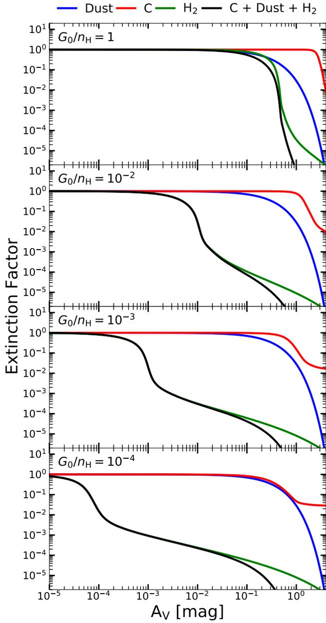
**Fig. B.2.** Extinction factor of dust in blue, of C in red, of  $H_2$  self-shielding in green, and of all of them combined in black, as functions of  $A_V$ . C I and  $H_2$  column densities are taken from Meudon PDR Code simulations for models with  $G_0/n_H = 1, 10^{-2}, 10^{-3}$ , and  $10^{-4} \text{ cm}^3$ .
