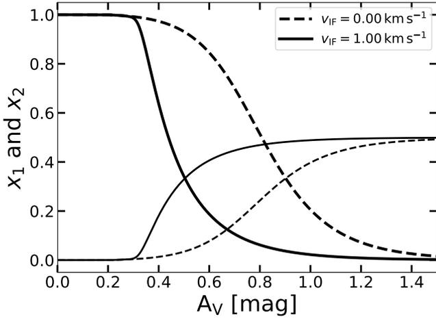
**Fig. 4.** Spatial profiles of H and H<sub>2</sub> abundances obtained by integration of Eq. (7) with typical PDR conditions, i.e.,  $G_0/n_H = 0.5 \text{ cm}^3$  and  $v_{\text{IF}} = 1 \text{ km s}^{-1}$ . The dashed lines are the static solution and the solid lines are the advection one.
