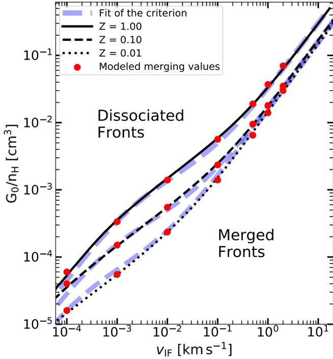
**Fig. 9.** Criterion describing, for a given ionization front velocity, the  $G_0/n_H$  ratio leading to a merge of the ionization and dissociation fronts. The red circles are the empirical merging values. The black lines are our new semi-analytical criterion from Eq. (15) and the blue dashed lines are the fits from Eq. (18). The ionization front and the dissociation front are merged to the right of the criteria.
