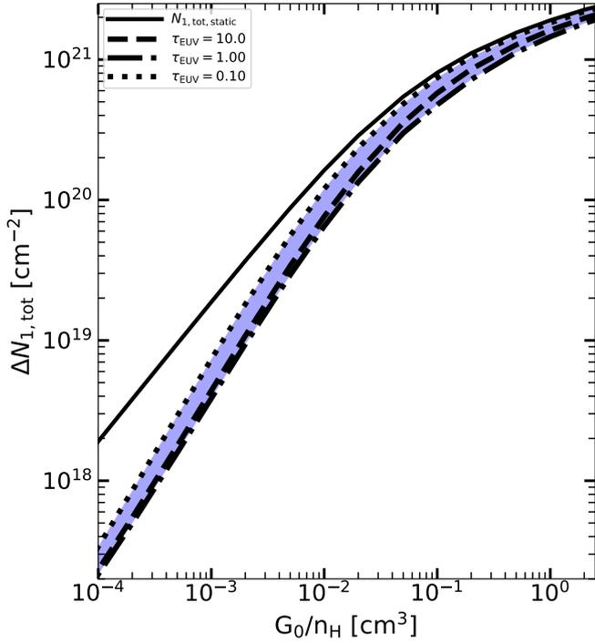
**Fig. 12.**  $\Delta N_{1,tot}$  range for different  $\tau_{EUV}$  compared with  $N_{1,tot}$  from the static solution, using the link between  $v_{IF}$  and the  $G_0/n_H$  ratio from Eq. (23). The closer  $\Delta N_{1,tot}$  is to  $N_{1,tot,static}$ , the stronger the dynamical effects.
