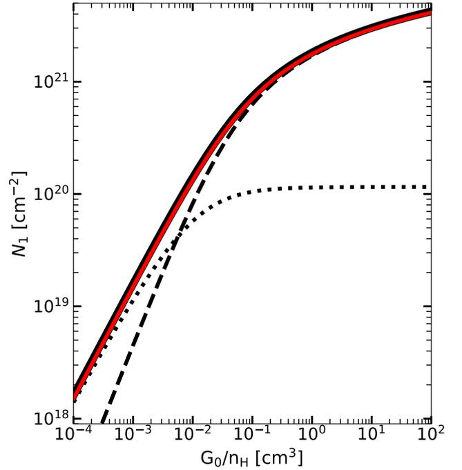
**Fig. 1.**  $N_1$  integrated over the atomic region (black dashed line),  $N_1$  integrated over the molecular region (black dotted line),  $N_{1,\text{tot}}$  (black solid line) as functions of  $G_0/n_H$  for a static and stationary approach, calculated by solving Eq. (8) analytically with Eq. (9). The red line is  $N_{1,\text{tot}}$  from Sternberg et al. (2014) calculated with a similar approach.
