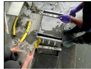
Submerged sediment trap
