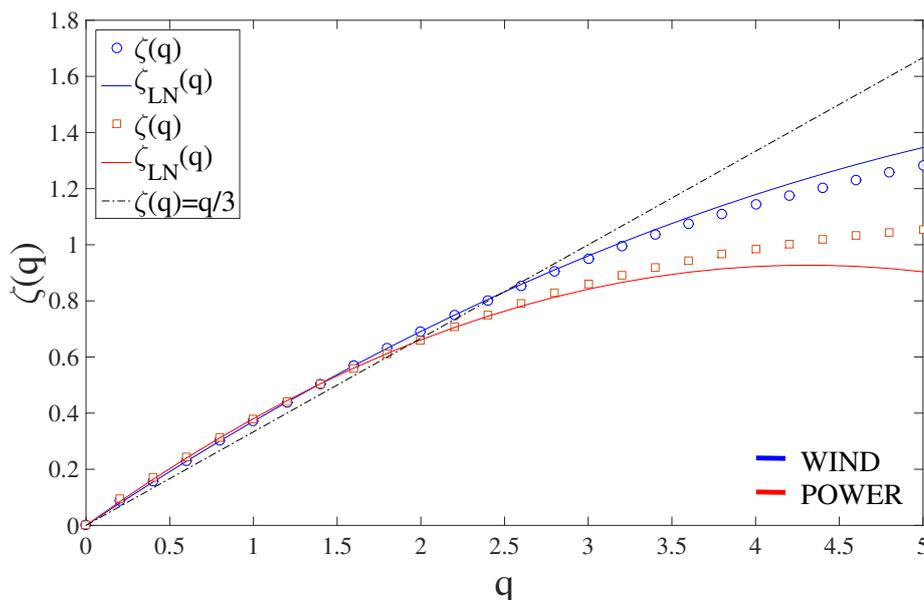
FIGURE 3 – The scale invariant moment function  $\zeta(q)$  estimated for wind and power output series coming from the turbine E-82. The log-normal models  $\zeta_{LN}(q)$  are superposed for each curve : the fit is respected for the lowest orders. The  $\zeta(q)$  functions are concave and compared to the linear function  $q/3$  (dashed line) which indicate the multifractal properties.
