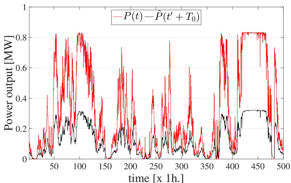
FIGURE 4 – Example of the forecast model applied to the E-44 turbine. This is a running forecast, with time  $t$  going from 0 to 500 and  $T_0$  fixed. The method is based on the long-range properties of invariant scale processes. The method has been applied during a period of 500 hours where the forecast horizon is  $T_0 = 10$  minutes and the learning window is  $T_1 = 166$  hours.
