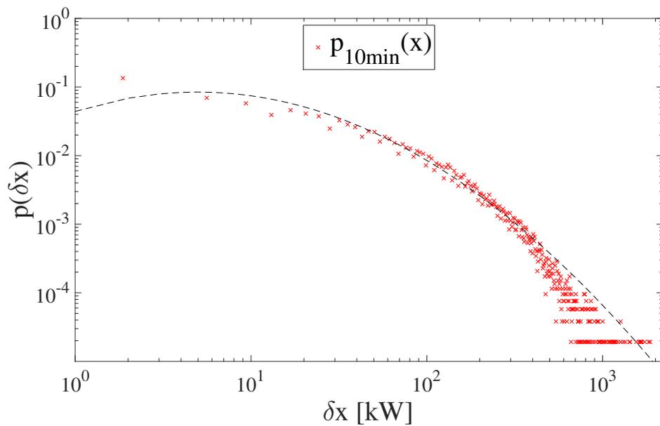
FIGURE 5 – Probability density function  $p(x)$  applied to the power output increments of the E-82 turbine at a time interval of 10 min. The log-normal fit (dashed line) is globally correct. Nevertheless, this adjustment does not capture power increments less than 20 kW and higher than 300 kW. The extremes are overestimated.
