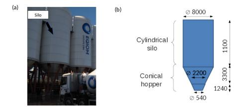
Figure 1: (a) Overview of the gravel silo of concrete facility and (b) the schematic of the gravel or sand storage silo (units in mm)
