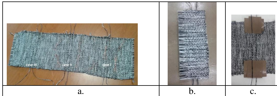
Figure 10: Textile sensors integration during weaving of 2D fabrics and its preparation for consolidation step: a) integrated textile sensors in 2D fabric, b and c) 2D fabric preparation for consolidation step
