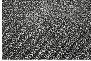
Figure 7: Thermoplastic powdered twill-weave fabric (Chomarat Composites)
