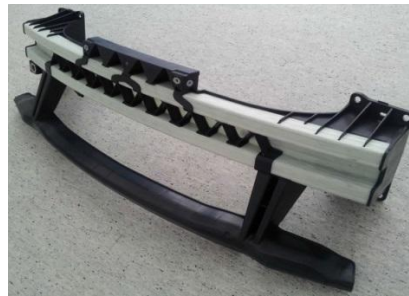
Figure 9: Front bumper crash beam produced with curved reactive thermoplastic pultrusion (Hyundai, Plastic Omnium, CQFD Composites and Arkema)
