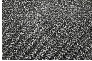
Figure 7: Thermoplastic powdered twill-weave fabric (Chomarat Composites)
