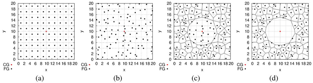
Figure 2 – Tessellation generation process: (a) initial seeds position, (b) seeds are randomly perturbed within a given region around initial positions, (c) and (d) seeds surrounding the CG are suppressed and subdivision is processed according to the weights assigned to each nucleus.
