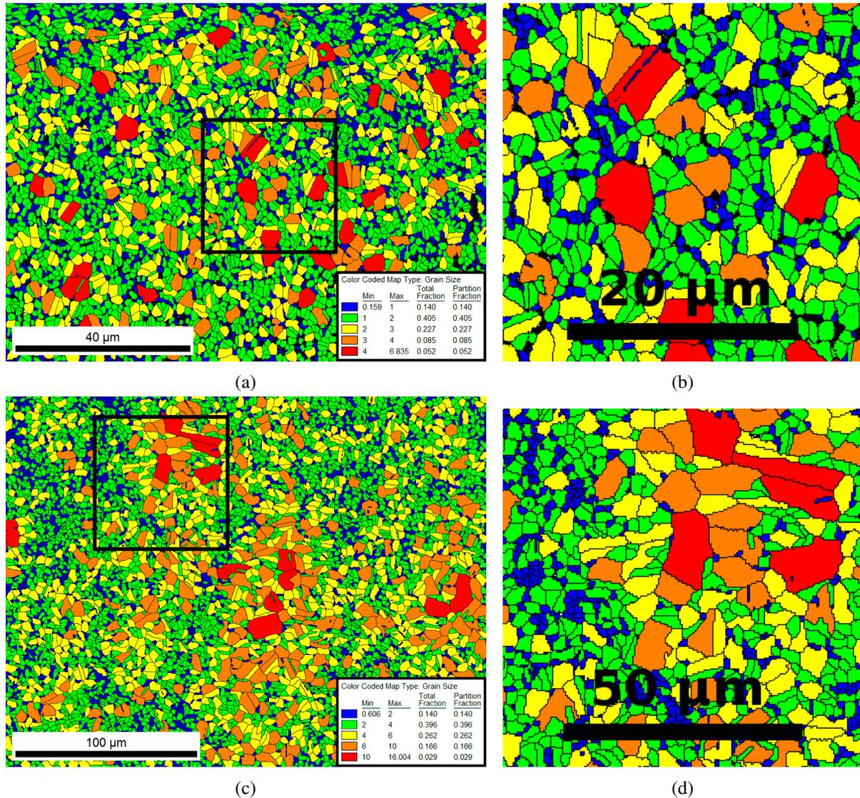
Figure 1 – (a) and (c) EBSD color maps based on grain-size for (a) a 50% CG - 50% UFG (volume fractions) blend of powder sintered by SPS and (c) a cold-rolled (up to 71% thickness reduction) sample and heat-treated at 850°C during 20 minutes. (b) and (d) provide zooms on the zones highlighted in (a) and (c).
