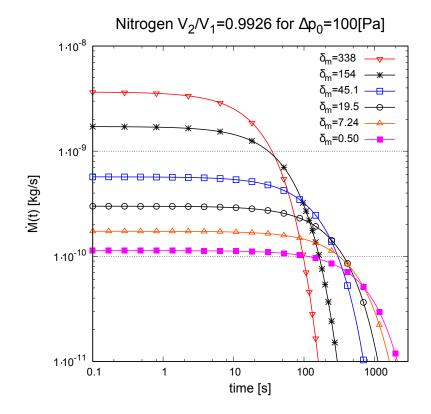
FIGURE 5 - Mass flow rate variation with time until a final equilibrium of no motion is reached through the tube for the same initial pressure difference.
