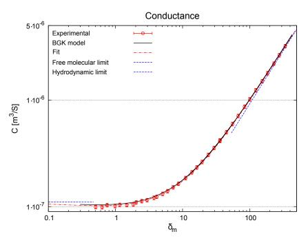
FIGURE 3 – Left : Exponential pressure difference variation with time  $\Delta p(t)$ .Right : Conductance ( $C = V_0/\tau$ ) for nitrogen ( $N_2$ ) as a function of the mean gas rarefaction conditions, that is from transition to near hydrodynamic regime.
