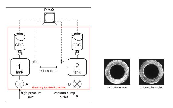
FIGURE 1 – The experimental apparatus composed by the micro-tube, two temperature sensors (t1 and t2), two tanks (R1 and R2) and the capacitance pressure diaphragm gauges (CDG). And details of the circular cross-section micro-tube.
