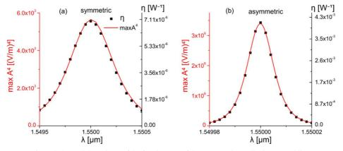
Figure 5: Spectral dependence of the fourth power of the pump mode amplitude at  $\omega$  (red line) and the SHG conversion factor (black squares) of the (a) symmetric (SYM) and b) asymmetric (ASYM) structures.
