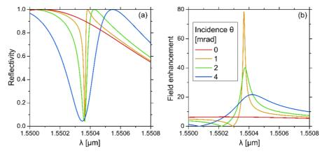
Figure 4: (a) The reflectivity spectrum of the infinite GC for different angles of incidence; (b) The corresponding electric field enhancement (with respect to the incident field) at the lower guide interface for a plane incident wave.
