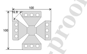
Figure 2: equi-biaxial tensile specimen geometry and dimensions.
