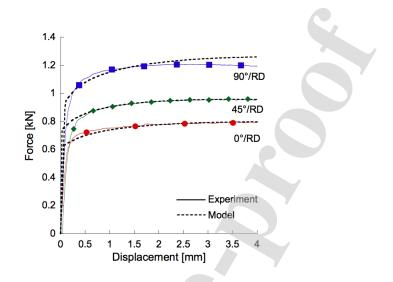
Figure 20: Comparison of force-displacement curves obtained by FE simulation and experimental tests for uniaxial tension along  $0^{\circ}/\text{RD}$ ,  $45^{\circ}/\text{RD}$  and  $90^{\circ}/\text{RD}$ .
