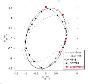
Figure 16: Yield surface description. Hill48(ref) corresponds to the model using material data parameters identified with  $(\sigma_0^0, r_0, r_{45}, r_{90})$ . Hill48 refers to the model using material data parameters identified with all experimental data. CB2001 is the yield surface obtained using Cazacu and Barlat's criterion [39].
