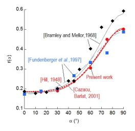
Figure 14: r-value prediction using  $(\sigma_0^0, r_0, r_{45}, r_{90})$  for the identification of F, G, H and N or the set of all experimental data (present work). The results obtained using the Cazacu-Barlat criterion [39] are also indicated. For comparison purpose, data from Bramley and Mellor [12] and Fundenberger et al [27] are provided.
