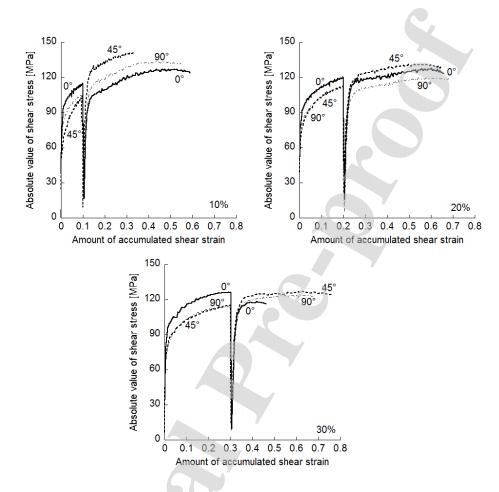
Figure 8: Absolute shear stress versus accumulated absolute amount of shear strain curve for simple shear loading.
