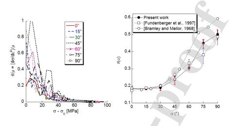
Figure 5: (a) Work-hardening vs amount of stress increase for different monotonic uniaxial tensile tests along different directions with respect to the rolling direction (b) Variation of r-value with orientation and comparison with data from literature on similar material
