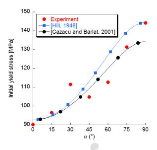
Figure 15: Initial yield stresses described using the Hill [5] and the Cazacu-Barlat [39] criteria
