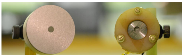
Fig. 5 Probes mounted on a rotation stage: (left) guard ring Faraday cup for the measurement of ion current and (right) gridded Faraday cup for the measurement of most probable ion energy.
