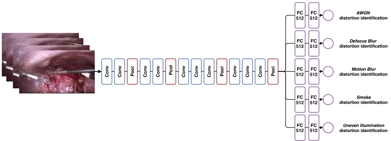
Fig. 3 Deep multi-task learning model for the classification of distortions in laparoscopic videos. Given an input video frame, our MTL model passes the frame through the CNN VGG16 to extract its most relevant features in the form of a vector that will be fed into the different classifiers, then each classifier (FC layers network) is fed with this vector to output a value indicating the probability of the presence of a specific distortion.
