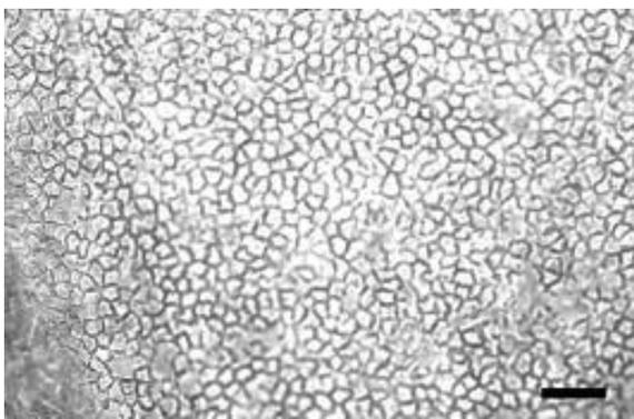
**Fig 2.** Image (0,1 × 0,1 mm<sup>2</sup>) of the endothelium of a cornea preserved in organoculture and observed under optical microscope after dilatation of the intercellular spaces by 0.9% NaCl (scale bar: 100 µm) (Laverne-Acquart, 2013).
