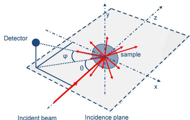
**Fig 3.** Definition of the measurement configuration.
