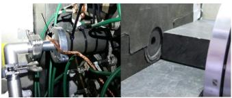
Fig. 4. Right: view of the front side of LOENIEv2 with a collimator aperture of 12 mm in diameter. One can see a part of the shielding wall made of borated polyethylene bricks. Left: view of the rear side of LOENIEv2 with a cylindrical shielding (5 mm of borated rubber) added for the <sup>233</sup>U campaign around the central tubing. The beam stop is placed in the iso-KF flange (see the arrow).
