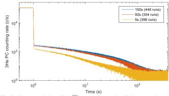
Fig. 8. Neutron emission of the  $^{239}$ Pu target in three irradiation scenarios (5 s, 50 s and 150 s of irradiation). No dead time correction was taken into account.
