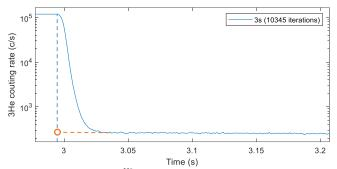
Fig. 7. Neutron emission of  $^{239}$ Pu in the case of short irradiation cycles (3 s of irradiation).
