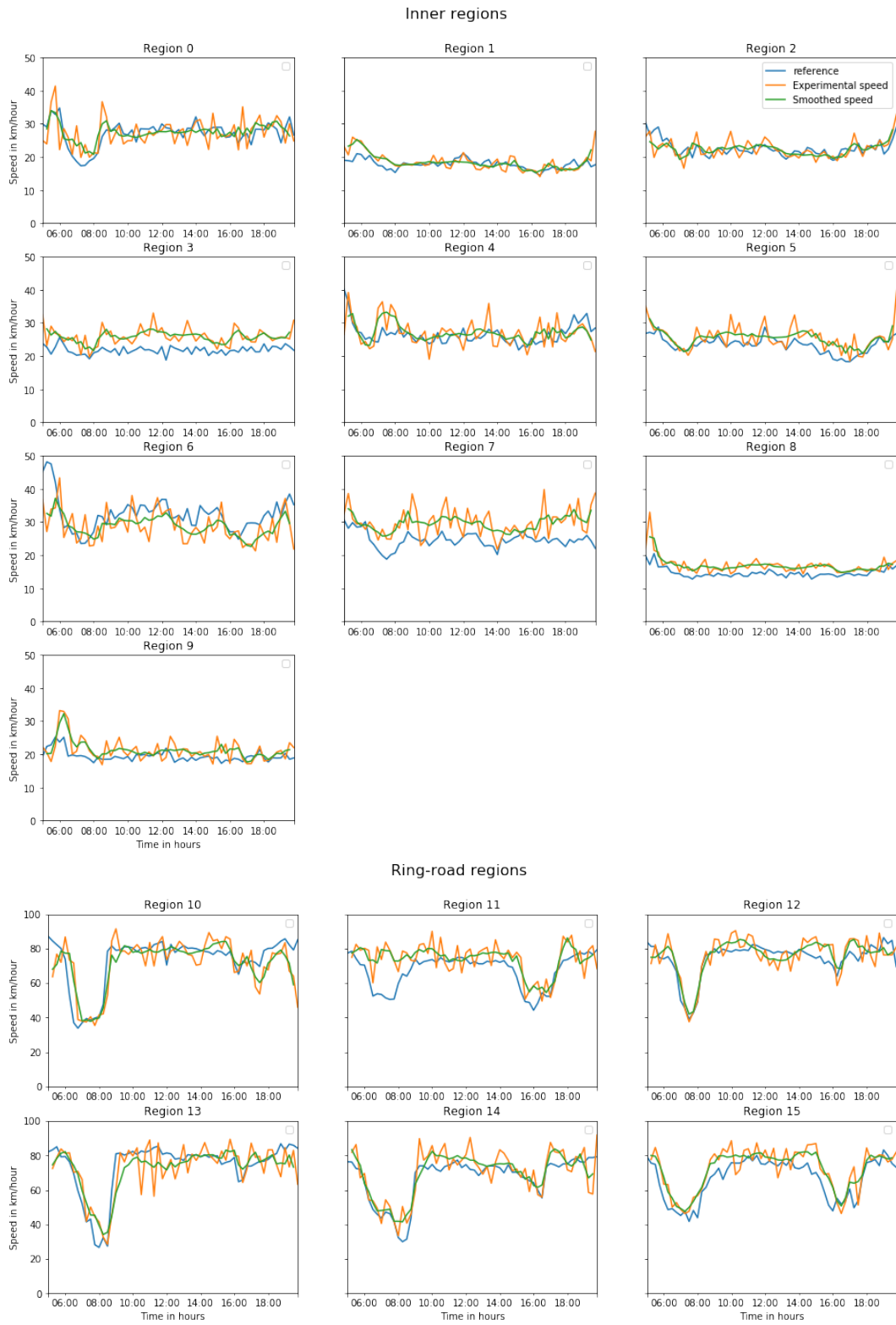
Figure 7: Speed estimation method applied to dataset DS_0 (trips with exact travel times), using the dynamic trip lengths
