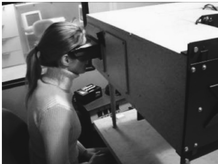
Fig. 18.2 A participant looking through a tachistoscope (three-channel Gebrandt T-scope) in the Shevrin lab (7 April 2009). The cards carrying the visual stimuli are individually lighted by neon light tubes at the side. Time and sequencing are monitored by a computer. © Ariane Bazan.
