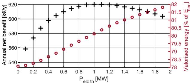
Fig. 6. Impact of electrolyzer power threshold  $P_{elz\ th}$  on the annual net profit (+ marker) and the valorised energy rate (o marker)
