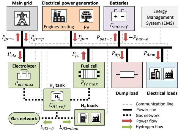
Fig. 1. Overview of the considered microgrid
