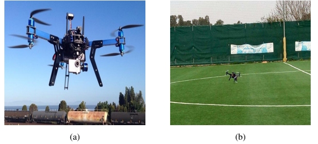
Figure 2: (a) 3D Robotics Y6 hexacopter [32] and (b) the Y6 drone in take-off phase.
