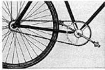
119. The chain drive on the old bicycle. (Photo by Carl Stein)
