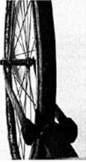
120. Front fork tubes are flattened for greater strength in their plane of stress. (Photo by Carl Stein)
