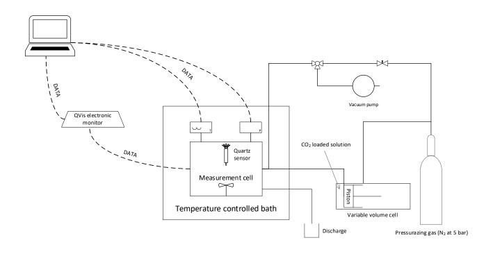
Figure 2: Scheme of the vibrating quartz viscometer (Flucon QVis 01/L) test bench.
