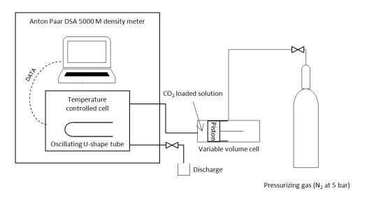
Figure 1: Scheme of the connection employed to charge the CO<sub>2</sub> loaded solvent in the Anton Paar DSA 5000 M density meter
