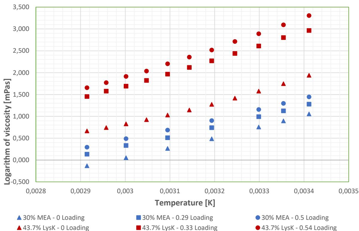
Figure 13: Experimental viscosity of CO<sub>2</sub> loaded 7 m MEA<sup>34</sup>(blue) and 4.21 m LysK (red) solutions at similar CO<sub>2</sub> concentration levels: 0( $\Delta$ ) – 0.29( $\square$ ) – 0.5( $\circ$ ) molCO<sub>2</sub>/molLysK.
