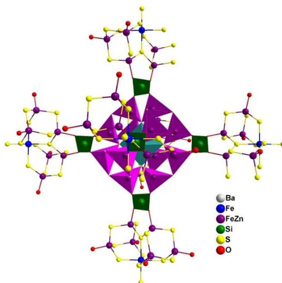
Figure 2. Representation of how clusters connect each other through the  $(\text{SiO}_4)$  groups.  $(\text{Fe}/\text{Zn})\text{OS}_3$ ,  $\text{SiO}_4$  and  $\text{FeS}_6$  polyhedra are represented respectively in purple, green and blue. Only the central cluster is fully represented to highlight the inter-clusters connection, Ba atoms are also omitted for clarity
